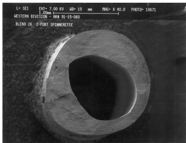
Figure 4 Hollow fiber membrane produced from two-port spinnerette using the design shown in Figure 3.
